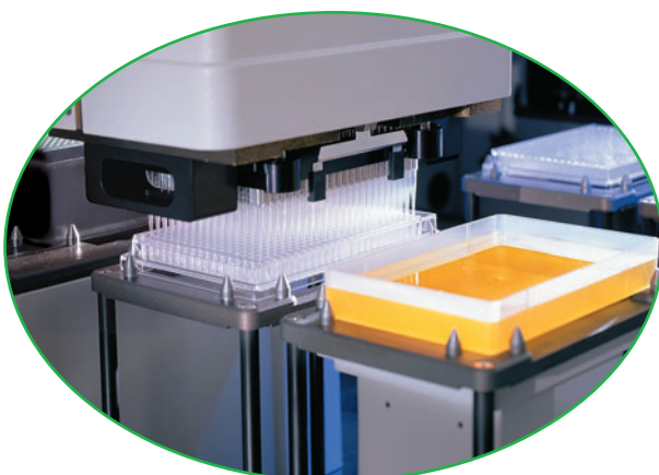
Biomek FX 384-Channel Disposable Tip Pipetting Head
